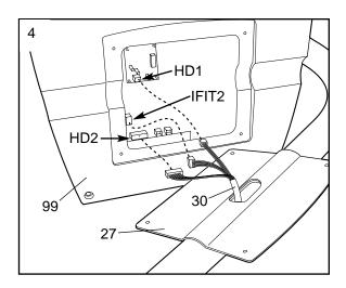
5. Attach the Console (99) to the Handrail (27) with the four Small Screws (6). Make sure that the Handrail Wire Harness (not shown) is not pinched between the Console and the Handrail.
